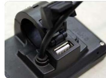
Each LCD Meter comes with a USB port attached to the bottom of the meter to charge your mobile devices. Hold down the [+] and set buttons for 2 seconds to turn on the USB charging. Hold the same buttons again for 2 seconds to turn this feature off.
