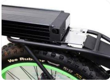
The battery must be mounted by sliding the fully charged battery forward onto the rear rack, over the rear wheel, through the channels on the battery while the carry handle is positioned at the rear. The key switch position must be in the “unlock” position to slide the battery on.
